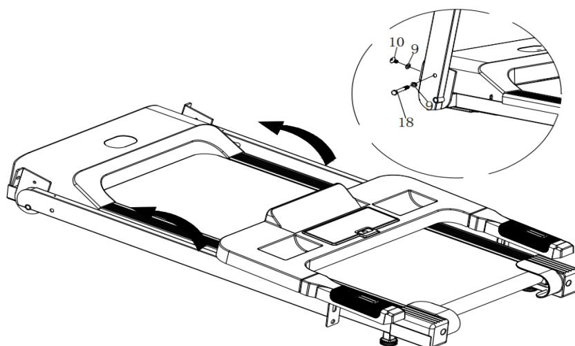
**STEP 2:** Use the M8x12 bolts (10) and washers (9) to secure the bracket to the front supports as described in the picture below.
